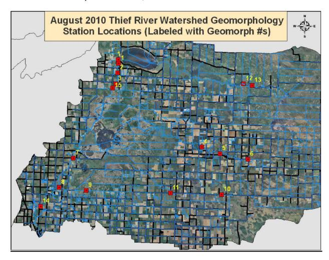
Each geomorphology site visit involved a reconnaissance of the reach, pool pebble count, riffle pebble count longitudinal pebble count, surveyed longitudinal profile, surveyed cross section profiles for the riffle and pool, establishment of a bank study site, bank erosion hazard index (BEHI) assessment at the bank study site, vegetation assessment, and monumenting of the cross sections.
